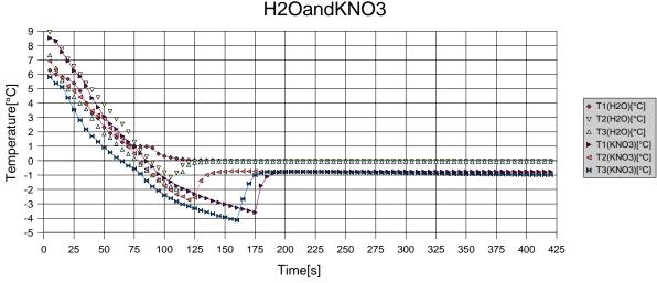
One can clearly see the different freezing points for distilled water and the KNO<sub>3</sub>-solution. Also, that the temperature of the water after reaching the freezing point stays constant meanwhile the temperature of the KNO<sub>3</sub>-solution slowly decreases (because the solution becomes more and more concentrated becausethesolventfreezesout)isclearlytobeseen.
