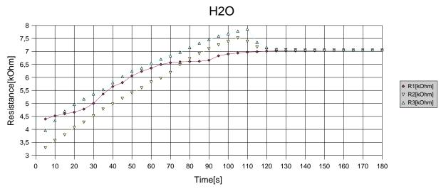
The graph of the first measurement does not reach a maximum; actually, this should not happen, maybe the temperature distribution was not homogeneous, so the thermistor did not measure the right temperature. Atthefollowing measurements, westirred more intensively, and it did not happen again.
