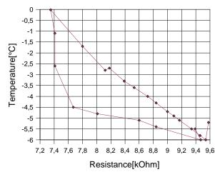
As one can see, some of our measurements are indeed crap. By taking only the measurements that lie on the lower-right end of the upper line of this diagram and by assuming a linear relation between resistanceandtemperature, we get the following function for the linear fit:
